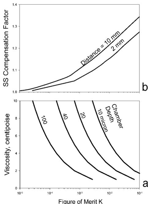
Figure 4. (a) Figure of merit as a function of viscosity and chamber depth for 2.0- $\mu\text{m}$ -radius spheres, surface tension 53 d/cm. (b) Predicted compensation factor from figure of merit  $K$  for distance 2 mm and 10 mm from point of entry.
