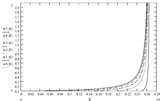
Figure 2. Computed trajectory of 4- $\mu\text{m}$ -diameter particles in capillary Poiseuille flow in a 20- $\mu\text{m}$  chamber.  $\beta$  (abscissa) is relative transverse location, and  $x$  (ordinate) is position in flow direction (mm from inlet). The lines indexed 0–5 correspond to initial value  $\beta = 0, 0.05, 0.1, 0.15, 0.2, 0.25$ , respectively. Segregation at SS plane  $\beta_0 = 0.265$  is almost complete after 1 mm.
