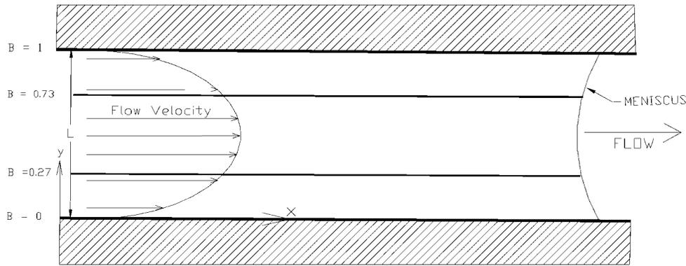
Figure 1. Capillary Poiseuille flow between 2 plates. Dimensions  $y$  is transverse,  $x$  is parallel to flow. Values of  $\beta$  given as  $B$ . The two SS planes are indicated at  $B = 0.27$  and  $B = 0.73$ .
