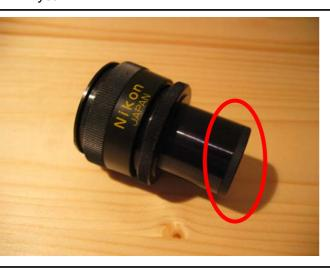
Step 1: Take your eye-piece out of the tube and unscrew the small ring at the lower end as indicated by the red eclips...
