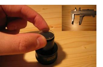
Step 3: Carefully place the supplied reticle in the eyepiece and replace the ring taken out during step 1.
